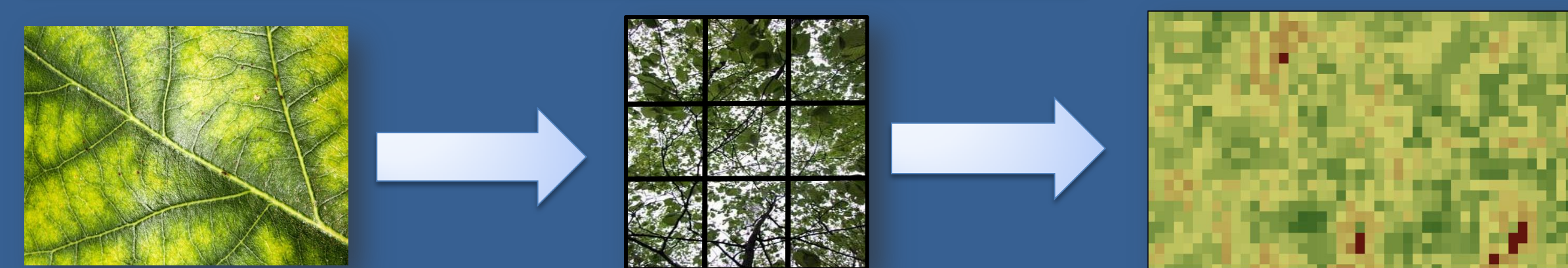
Figure 5: Maps of canopy nitrogen (N) are created using a scaling process that goes from the leaf-level to the plot-level and then to the canopy-level. The process begins in the field, where representative species are sampled and transported back to the lab. Percent N values are derived using a CNS analyzer and then scaled to the plot-level using estimates of species fractional proportion. Partial least squares (PLS) regression relates these plot-level values with AVIRIS reflectance values to create maps of canopy N across broad spatial scales.
