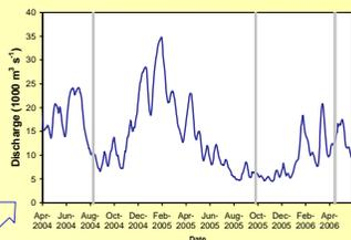
Fig. 3. Mississippi River stage determined at Baton Rouge, LA (data courtesy of USGS). Gray lines indicate cruise periods. River stage is typically high in spring and early summer and declines into the fall.
