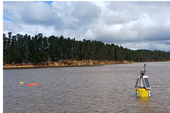
BioSCape deployed first hyperspectral radiometric buoy in Africa.
