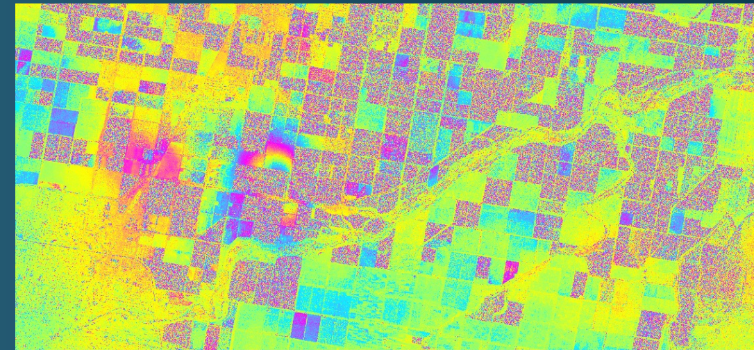
22-day pair in S. California, showing coherence and signals in agricultural fields and clear signal at geothermal plant.
